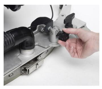
the machine: install and fasten it with the handwheels, then connect to the suction hose.
