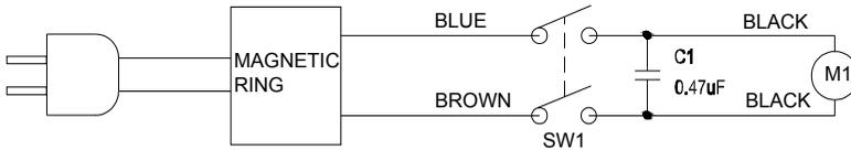
**Wiring diagram for VL100 55L/75L(figure10)**
